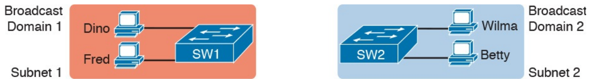
Figure 1-1 Creating Two Broadcast Domains with Two Physical Switches and No VLANs
