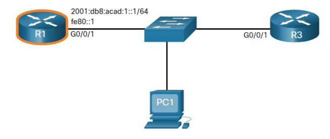
In this example, R1 will provide SLAAC services for the host IPv6 configuration and DHCPv6 services.
